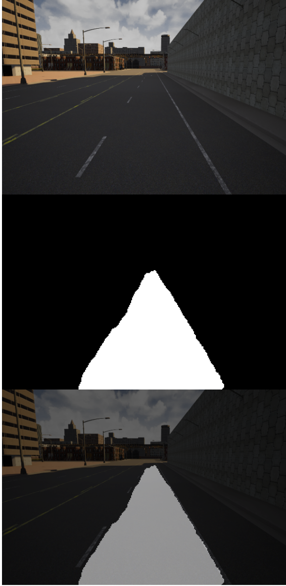
Fig. 6. Lane segmentation input image, binary segmentation mask and overlay for visualisation
