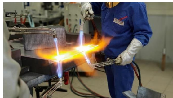
Figure 1: Manual bending of quartz glass [1]
