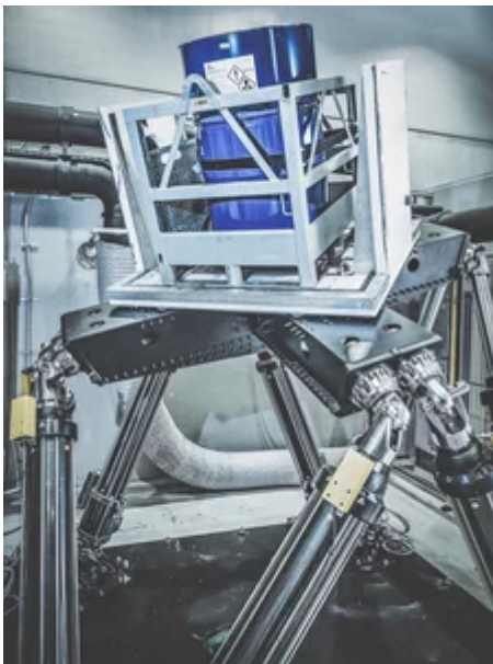
Electrical movement platform on eight legs (octopods)
